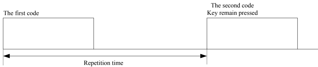
Figure 10-9 RC5 Protocol of Repetition time
